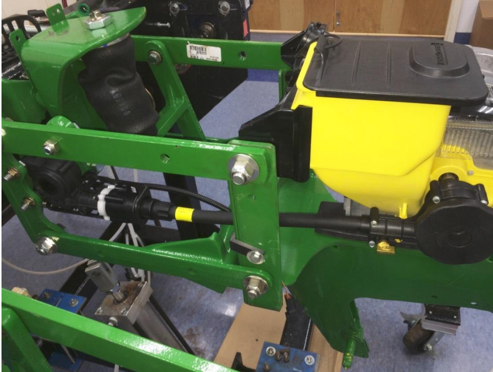
Finished Gearbox and Shaft Install
