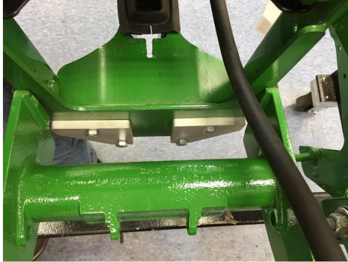
Row stops installed.
